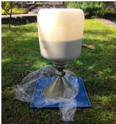
c. Kerucut pasir (*sand cone*)
