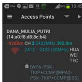
Figure 4. Example of the Wi-Fi Signal Strength Measurement Interface at Test Point TU5
