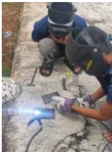
Figure 5. Welding Training by Joining Two Metals
