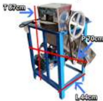
Figure 1. Aloe Vera Peeling Machine with Specifications 70 cm x 44 cm x 87 cm
