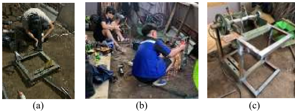
Figure 4. (a) Material Cutting, (b) Welding and (c) Painting
