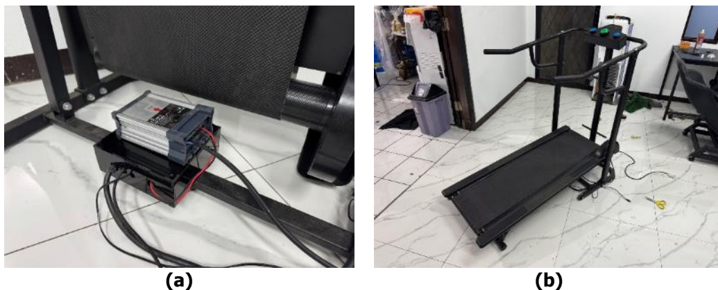
Figure 3. Physical Setup of the Developed System: (a) Electronic Module Enclosure and PSU Installed Underneath the Treadmill; (b) Complete Embedded System Integrated with the Manual Treadmill Structure
