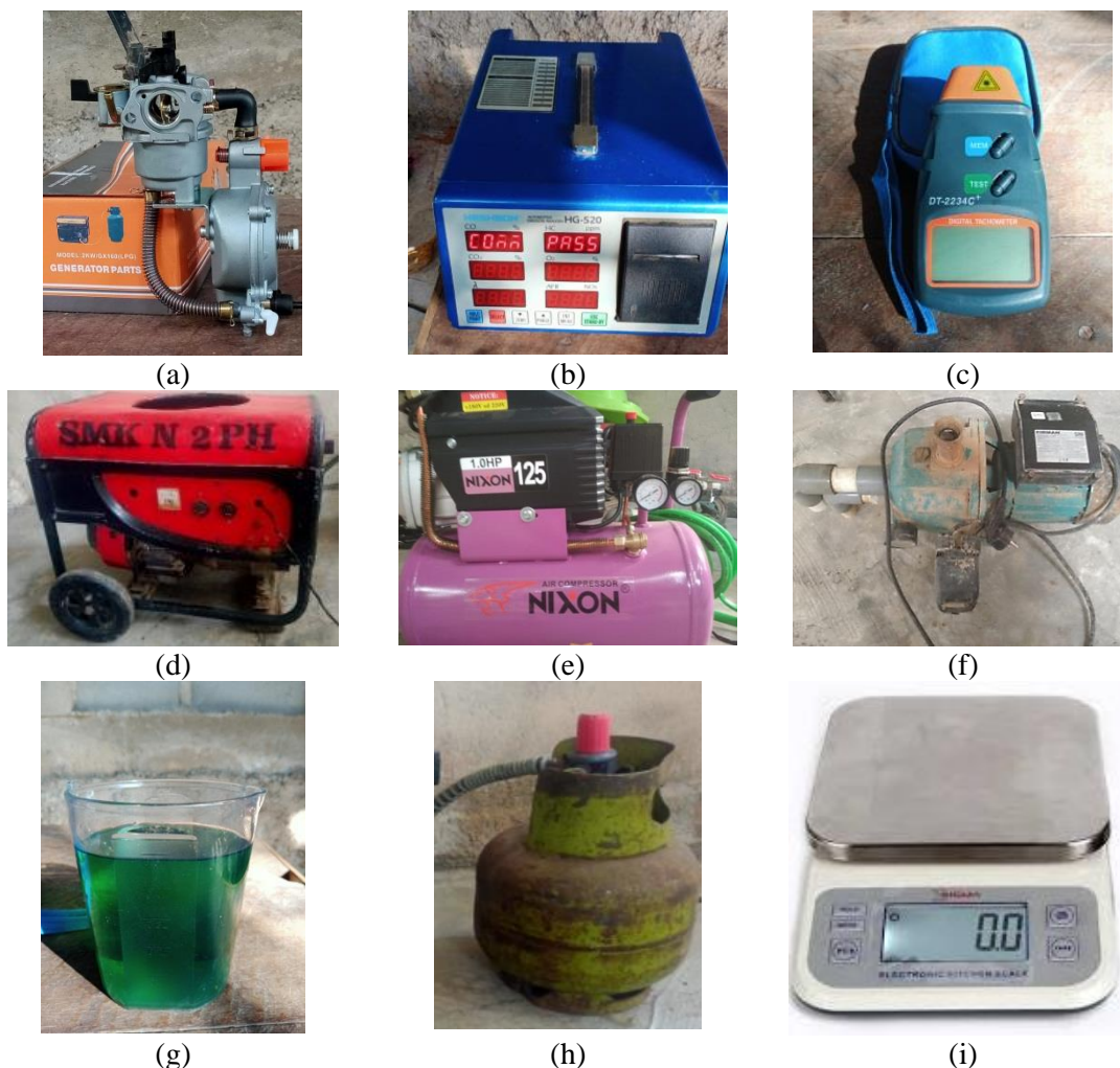
Gambar 2 Alat dan Bahan (a) Vacuum Converter; (b) Gas Analyzer; (c) Tacho Meter; (d) Genset Honda GX 160; (e) Kompresor; (f) Pompa; (g) Pertalite; (h) Gas LPG; (i) Timbang
