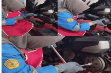
Gambar 1. Melepas Cover, Melepas pully belakang ( Driven Pully )
