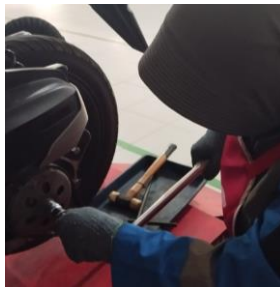
Gambar 3. Memasang kembali pully belakang ( Driven Pully )
